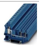
Feed-through terminal block, Connection method: Screw connection, Cross section: 0.5 mm<sup>2</sup> - 16 mm<sup>2</sup>, AWG: 20 - 6, Width: 10.3 mm, Color: blue, Mounting type: NS 35/7,5, NS 35/15
